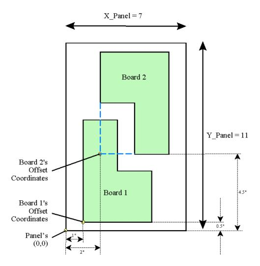
Looking at the figure, which shows the panel (with the Primary side facing you), obtain the X\_Offset and the
