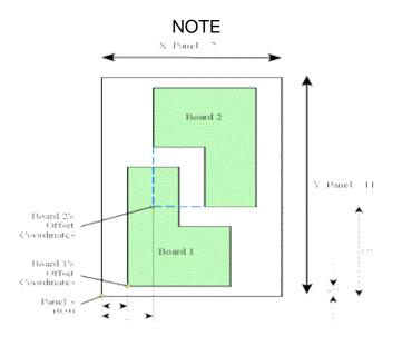
Since the boards are L-shaped, the corner is a virtual point. If the board had been rectangular, then the point would be the actual corner of the board.
